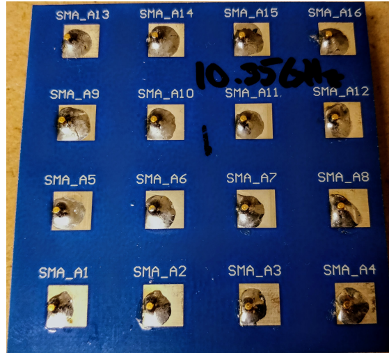
Figure 3.7: A working prototype board of the 4x4 patch antenna design.
